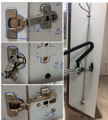
Fig. 5. Three-hinged MDF door after test
