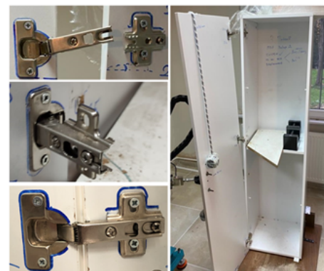
Fig. 6. Three-hinged PB door after test
