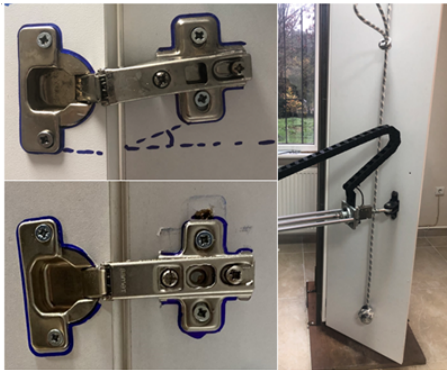
Fig. 3. Two-hinged MDF door after test
