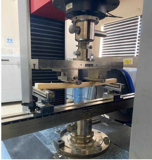
Fig. 5. Performing flexural strength and modulus of elasticity test
