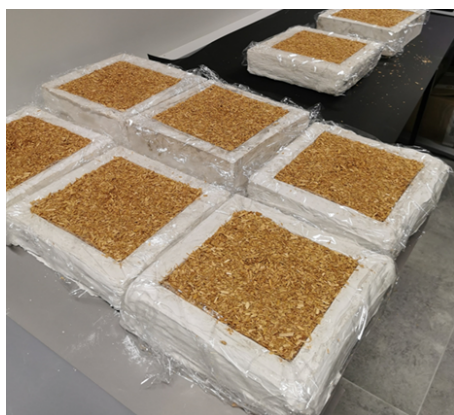
Fig. 1. Wall cladding element before ripening – the form is filled with MBC material (photo by A. Bonenberg)
