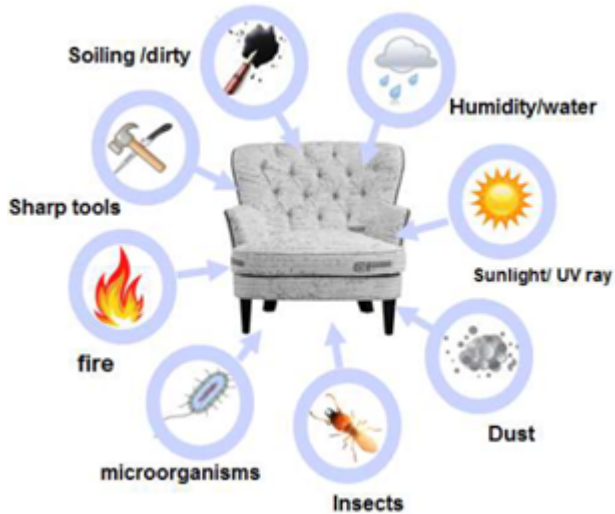
Fig. 1. Some of the factors that lead to furniture damage (Mahr, 2019)
