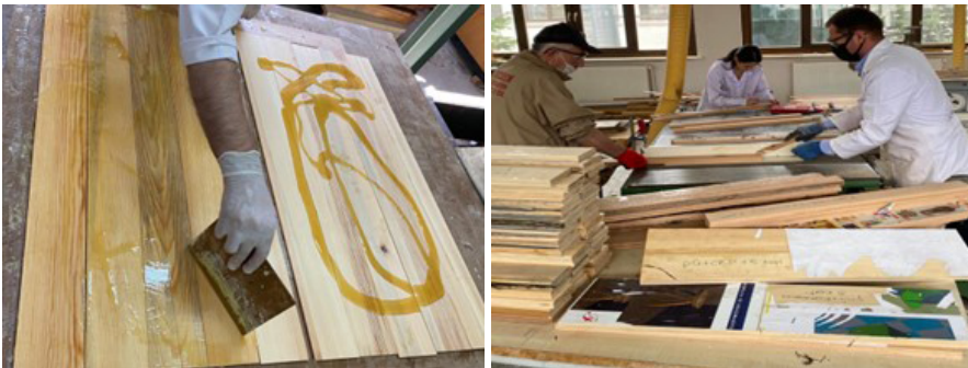
Fig. 2. Preparation of the test samples
