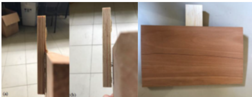
Fig. 11. Failure modes of the joints: a) shear among the layers of gusset-plate; b) separation from connection points; c) main member rupture
