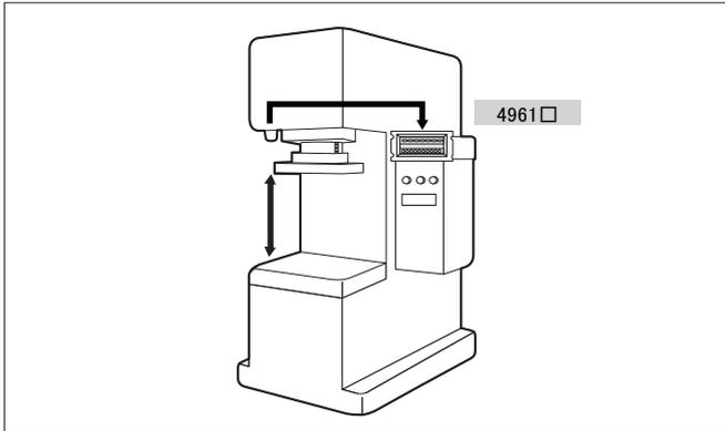
As in the figure on the left, when the press machine finishes operation and returns to the upper edge, the adjacent switch is activated. To display the operating time of the press machine (when the proximity switch is turned off)
