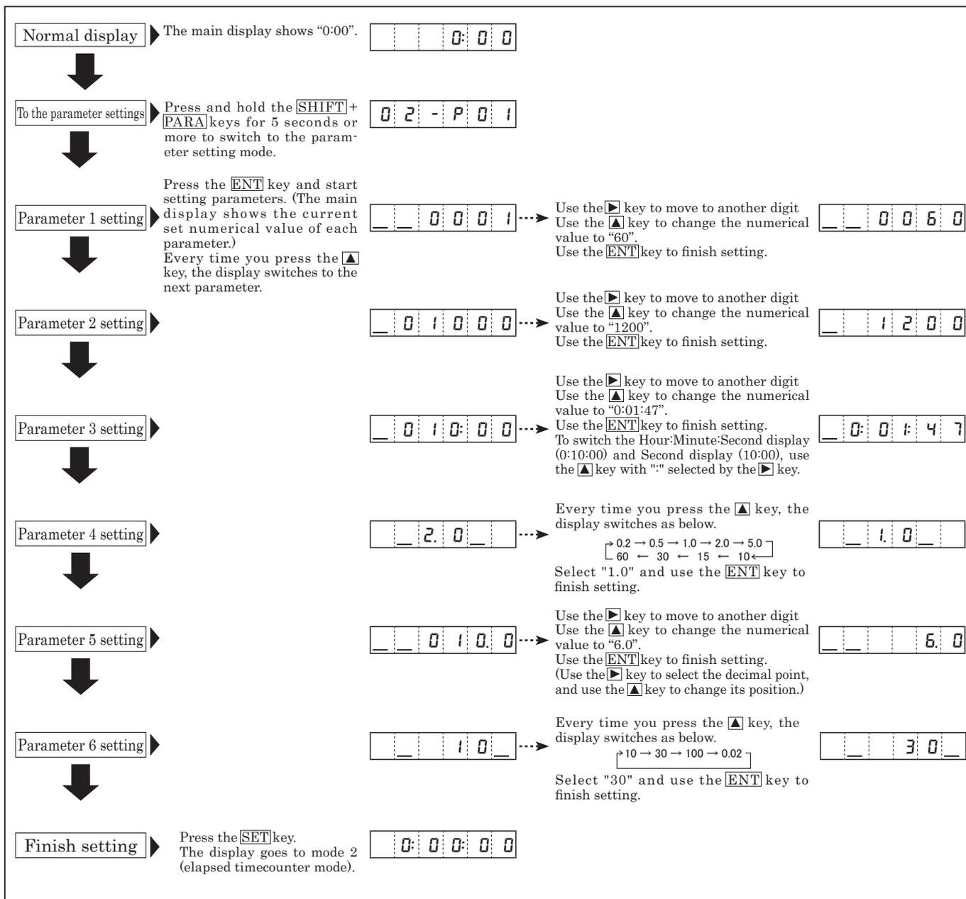
\*If you enter a value outside the setting range, all the input values will blink, which indicates the setting is disabled. When this occurs, you cannot switch to other displays until you enter a value within the setting range.
