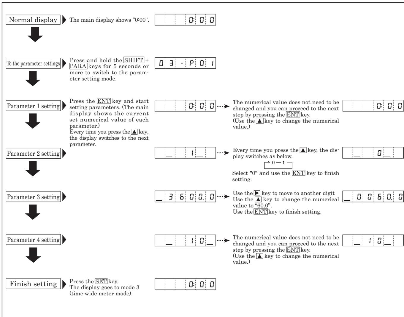
\*If you enter a value outside the setting range, all the input values will blink, which indicates the setting is disabled. When this occurs, you cannot switch to other displays until you enter a value within the setting range.
