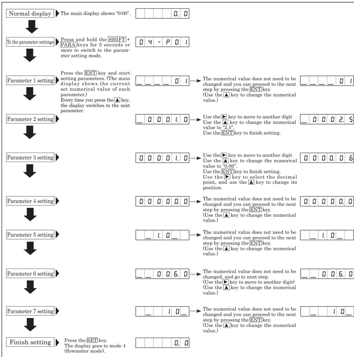
\*If you enter a value outside the setting range, all the input values will blink, which indicates the setting is disabled. When this occurs, you cannot switch to other displays until you enter a value within the setting range.
