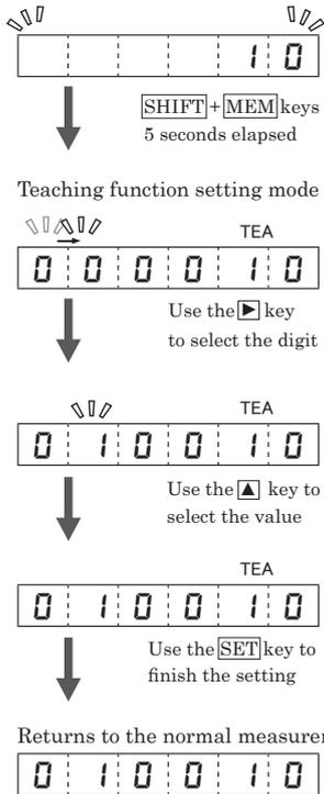
When you press the **[SHIFT]** + **[MEM]** keys simultaneously during the normal measurement display, the main display blinks. (TEA lamp lights up)
