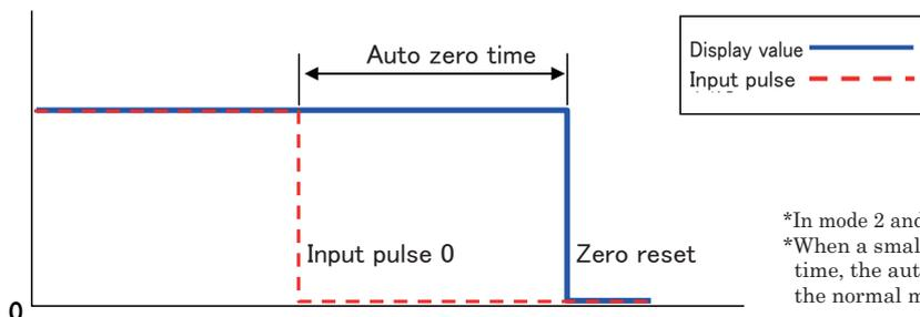
\*In mode 2 and mode 3, the zero reset display is "----".
