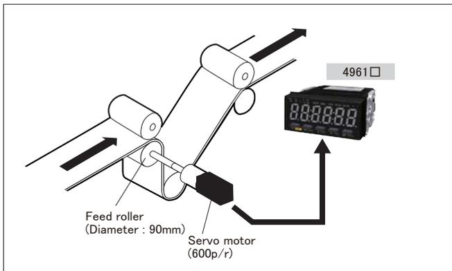
As in the figure on the left, the rotary encoder is connected to the feed roller via coupling in the paper manufacturing process. To display the peripheral speed (m/min.) of the feed roller in 4961□ under the following conditions:
