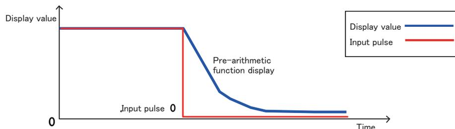
When the auto zero function is activated, the display becomes “0” (“-.-.-.-.-” in mode 2 and mode 3).
