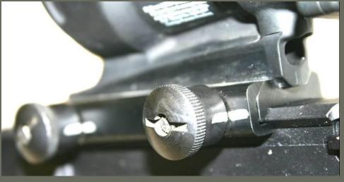
Mark Thumb Screw location with permanent marker or other means.
