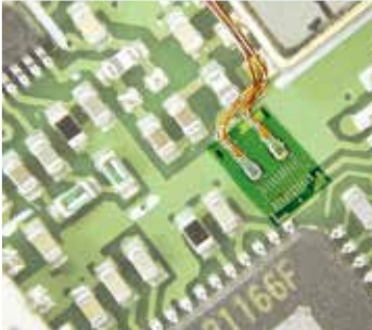
Strain gauges on printed circuit board
