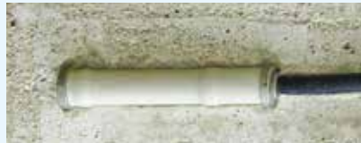
Full bridge Strain Transducer KM series
