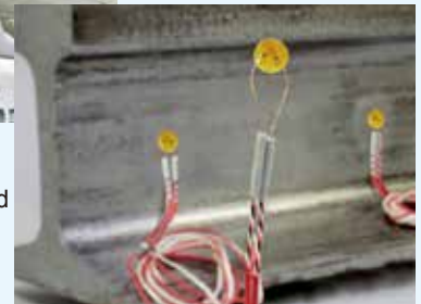
Strain measurement less influenced by EM noise between pantograph and trolley wire of electrified railway system
