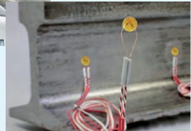
Railway axle load measurement
