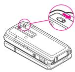
Pull out Battery Cover Latch as shown in ①, then slide cover as indicated in ②
