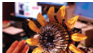
Himawari Plant Robot: Creature Expression Using Shape-Memory-Alloy Actuator Cluster
