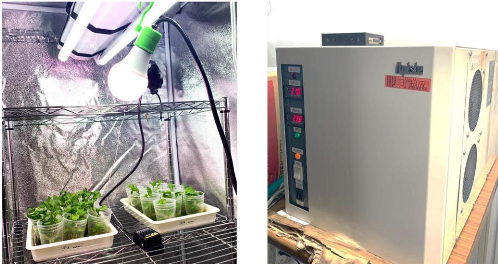
Figure 1. A custom-made growth chamber (left) with the temperature and humidity controller (right).
