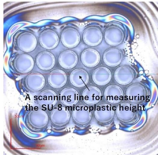
**Figure 6:** A confocal laser microscope image of the SU-8 microplastics with a scanning line.
