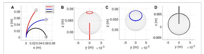
FIGURE 10 | Position redundancy evaluated for three positions for a FAS segment. (A) Three configurations considered for evaluation. The service sphere is plotted for configuration one in red (B), two in blue (C), and three in black (D). Friction coefficient is assumed to be zero.
