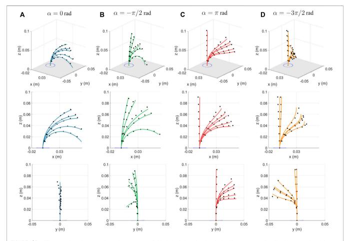
**FIGURE 6** | For different tension values, experimental measurements (in black dots) plotted against the backbone curve predicted by the proposed model for **(A)**  $\alpha = 0$ , **(B)**  $\alpha = -\pi/2$  rad, and **(D)**  $\alpha = -3\pi/2$  rad. The figures show the 3D plot (top row), projection on the xz-plane (middle) and the projection on the yz-plane (bottom).
