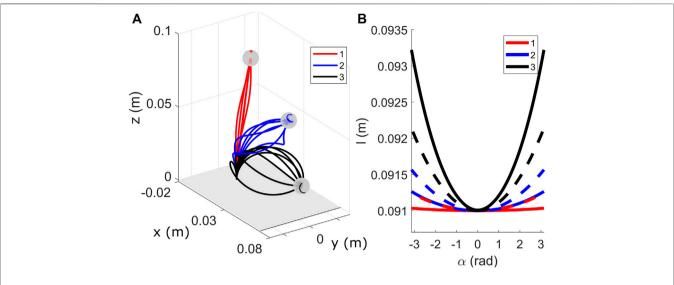
**FIGURE 11** Variation in redundant robot configurations (**A**) Sparse redundant configurations with  $\mu = 0.3$ , for the same tensions considered in **Figure 10** (**B**) Plot of variation in length of the backbone with  $\alpha$ . The dashed lines represent the plots for  $\mu = 0.3$  and solid lines for  $\mu = 0.3$
