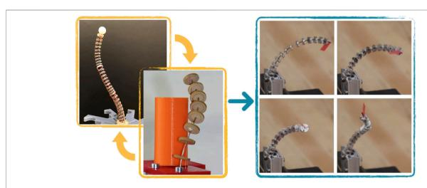
FIGURE 1 | Envisioned tendon-driven continuum robot (on the right) as combination of extensible segment TDCR [top left, from (Amanov et al., 2019)] and TDCR with helical routing [bottom left, from (Starke et al., 2017)].
