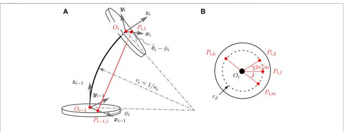
**FIGURE 4 | (A)** Diagrammatic representation of two disks *i* and *i* – 1 and the portion of the backbone between them. The corresponding frames attached at  $O_{i-1}$  and  $O_i$  have been indicated. Only one tendon has been marked red for clarity. **(B)** The *m* tendons are arranged concentrically around the backbone at a distance of  $r_{cl}$ .
