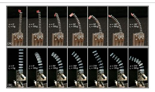
**FIGURE 3** | TDCR prototypes. Both prototypes are loaded with different weights on one tendon for different rotation  $\alpha$ . **(A)** First prototype is composed of type-III FSD with fixed overall length of 60 mm. **(B)** Second prototype is composed of type-II FSD.
