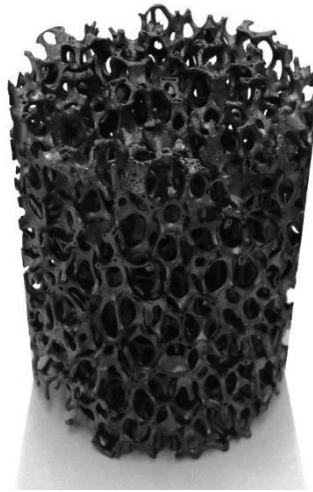
Figure 7-2: Structure packing made of 10 ppi SiSiC reticulate porous ceramic (RPC) foam installed in the solar gasifier. Image from [88].
