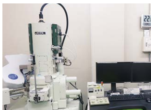
▲電界放出形走査電子顕微鏡 (EDS/WDS/EBSD付) Field Emission Scanning Electron Microscope (equipped with EDS/WDS/EBSD)
