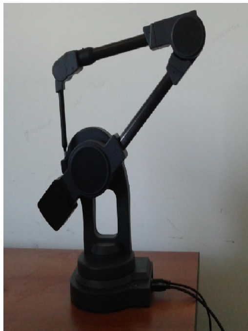
Figure 2. The MicroScribe-Gx device used in measurements
