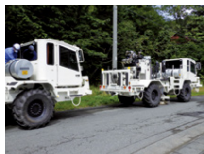
Fig.3 Seismic survey of supercritical geothermal systems
