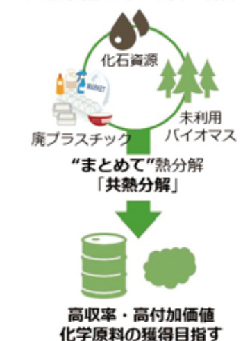
Fig.4 Highly efficient utilization of carbon resources by the control of pyrolytic synergistic interactions during co-pyrolysis
