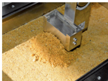
Fig.2 Blade excavation experiment
