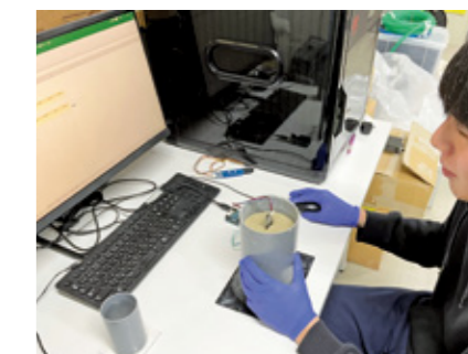
Fig.6 Experiment to measure water content in the soil
