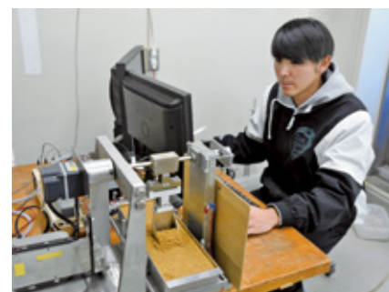
Fig.1 Apparatus for bucket excavation
