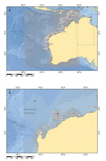
Figure 2.3 Hydrodynamic model grid (grey wire mesh) used to generate the tidal currents, showing locations available for tidal comparisons (red labelled dots). The top panel shows the full domain in context with the continental land mass, while the bottom panel shows a zoomed subset near the discharge locations. Higher-resolution areas are indicated by the denser mesh zones.
