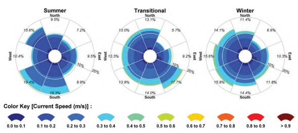
Figure 2.2 Seasonal current distribution (2006-2015, inclusive) derived from the BRAN database near to the proposed FPU location. The colour key shows the current magnitude, the compass direction provides the direction towards which the current is flowing, and the size of the wedge gives the percentage of the record.
