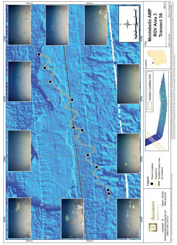
Figure 3-14 Typical benthic habitat and bathymetry in Area 3a.
