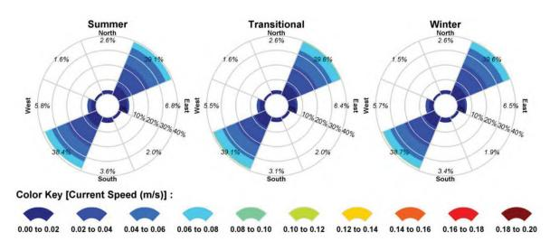
Figure 2.6 Seasonal current distribution (2006-2015, inclusive) derived from the HYDROMAP database near to the proposed FPU location. The colour key shows the current magnitude, the compass direction provides the direction towards which the current is flowing, and the size of the wedge gives the percentage of the record.
