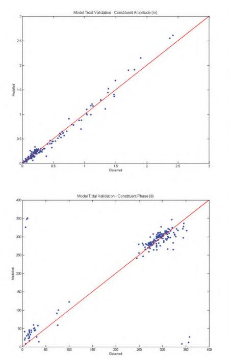
Figure 2.5 Comparisons between modelled and observed tidal constituent amplitudes (top) and phases (bottom) at all stations in the HYDROMAP model domain. The red line indicates a 1:1 correlation between the modelled and observed data.
