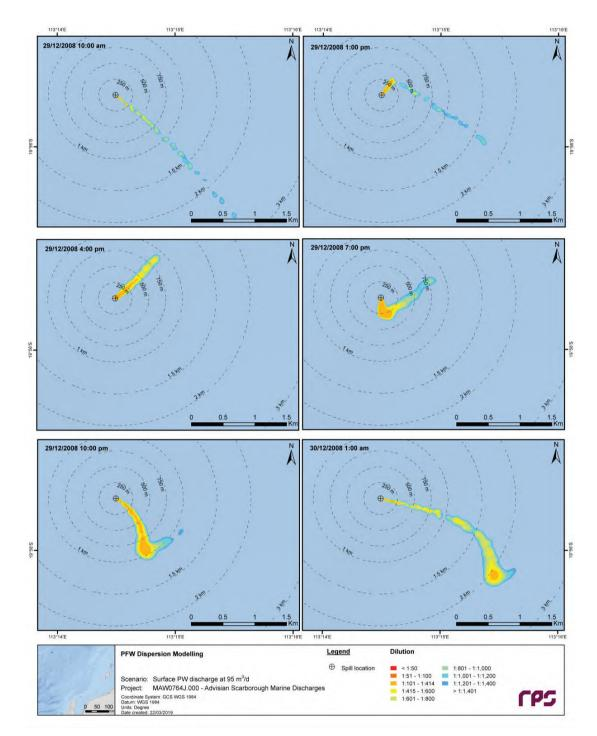
Figure 3.13 Snapshots of predicted dilution levels, at 3-hour intervals from 10:00 on 29<sup>th</sup> December 2008 to 01:00 on 30<sup>th</sup> December 2008, for Case P1 (0 m depth discharge at 95 m<sup>3</sup>/d flow rate).
