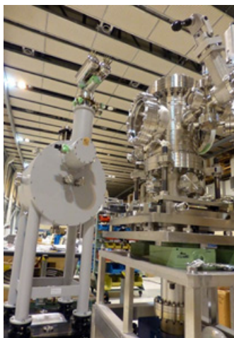
Fig. 4. Soft X-ray MOKE station
