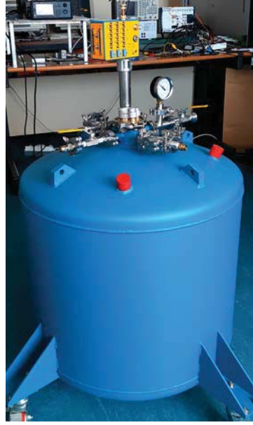
Fig. 1. Photograph of the dewar with the short cryoprobe inserted end equipment to ensure safety operation during its use.
