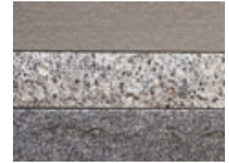
Treads Top: Bluestone Middle: Salt and Pepper Granite Bottom: Blue Mist Granite
