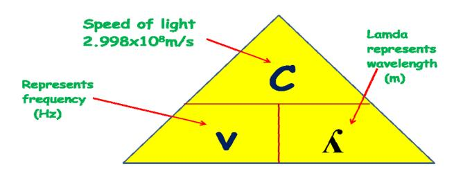
V = frequency; C = speed of light;  $\Lambda$  = wavelength Hz (waves/s) 2.998×10<sup>8</sup>m/s metres (m)
