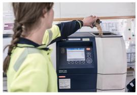
The Infratec™ 1241 is a whole grain analyser using near-infrared transmittance technology to test multiple parameters such as moisture, protein, oil, starch etc. in a broad range of grain and oilseed commodities.
