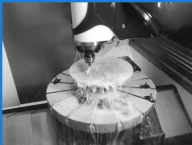
Manufacturing of cooling channels
