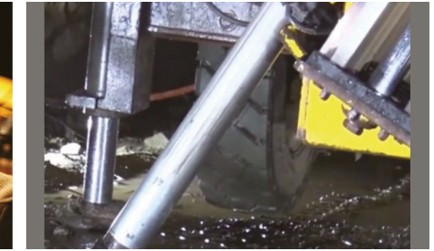
Sturdy stingers on front and rear to support drilling in steady position, that increases accuracy of drilling and decreases consumption of drill string.
