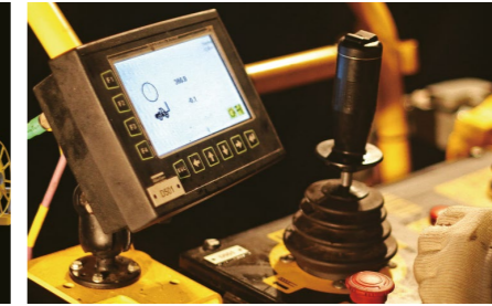
Digitized angle reading system helps operators to fulfill more accurate hole angle and depth.
