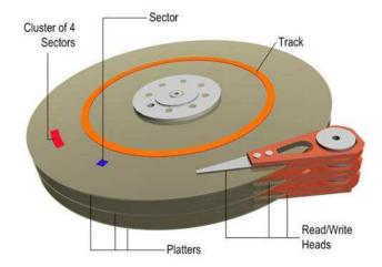
**Sector**: also called a **disk block**, a series of consecutive bits along a track. Every sector has a unique logical disk address called CHS: cylinder-head-sector. A sector is the smallest **addressable** unit of storage on the disk. A common size is **512 bytes**. Some older documentation uses the term "sector" to refer to all sectors on all tracks within a specific pie shaped wedge. In this terminology, the disk block is the intersection of a track and a sector.
