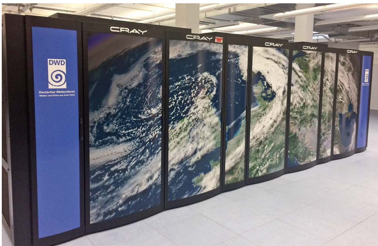
Figure 18: Mainframe computer of the DMRZ (CRAY-XC40) in Offenbach. The computer is operated by the DWD; the Bundeswehr's share of the computing capacity is 20% (source: DWD).
