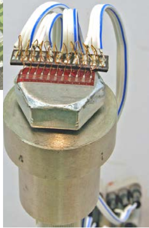
10-element chain type strain gauges on bolt head
