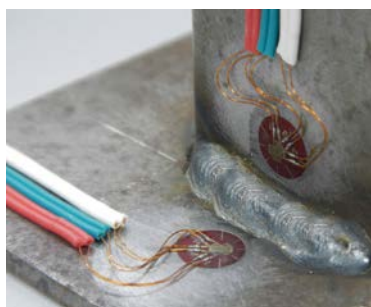
Weld bead (rosette strain gauge)
