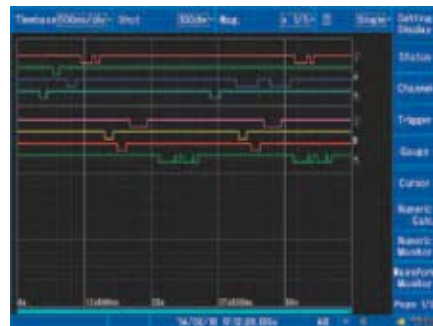
• Multi-channel timing measurement using logic waveform measurement
