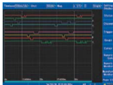
• Multi-channel timing measurement using logic waveform measurement
