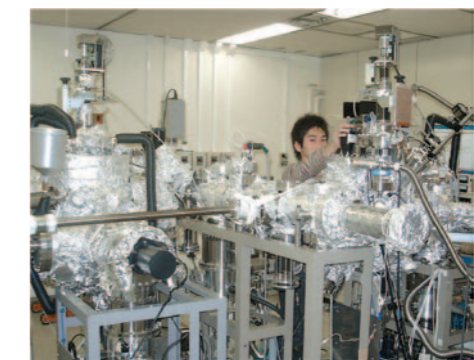
■ 超異種基板上のヘテロエピタキシャル成長を実現するユニバーサル成長装置 Universal epitaxial chambers which make it possible to grow semiconductor films on various substrates with large lattice mismatches.
