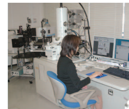
■ 電子線励起による発光、回折、電流等を測定する複合分析装置 Characterization tools which detect luminescence, electron diffraction, and current induced by electron beam irradiation.
