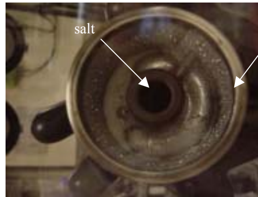
FIG. 14. Recovered salt and Cd by cathode process.
