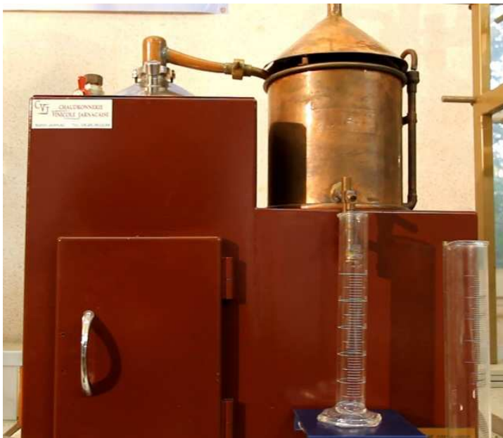
Figure 3. Laboratory-scale Charentaise style still used for production of eau de vie (photo courtesy of Conservatoire du Vignoble Charentais).
