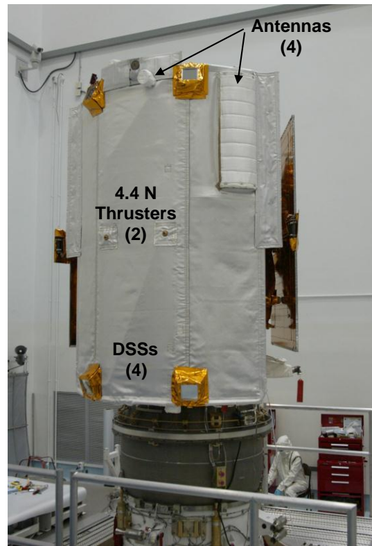
Figure 3. Shown is the MESSENGER spacecraft 2 weeks before launch. Highlighted here are the ceramic-cloth sunshade, the four DSSs with attenuating filters, the phased arrays and low-gain antennas under high-temperature radomes, and the 4.4-N pro-Sun thrusters.
