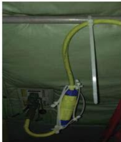
Figure 6.3. KC-135 Pigtail adaptor (P/N 8564034-135).
