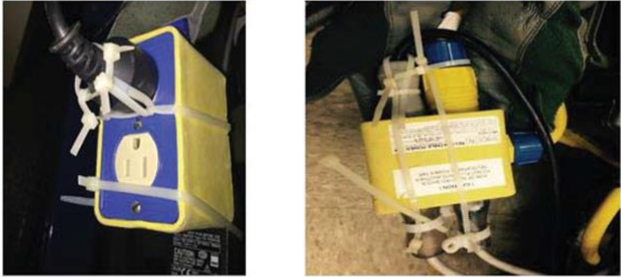
Figure 6.3. KC-135 Pigtail adaptor (P/N 8564034-135).
