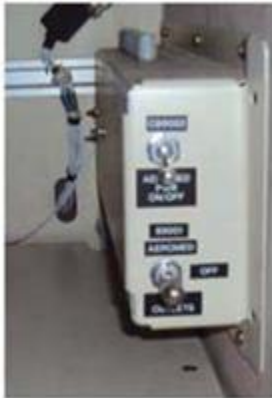
Figure 8.1. Aero Medical Master Control Panel.
