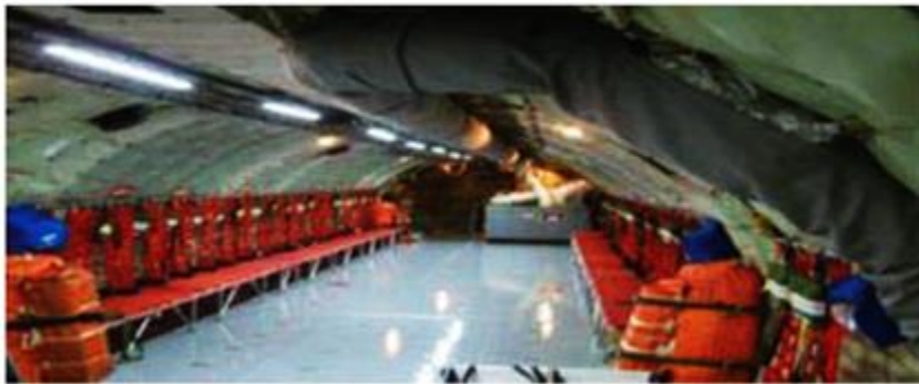
Figure 6.4. Portable Cargo Lighting System.
