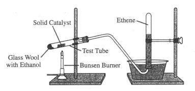
Ethene, C<sub>2</sub>H<sub>4</sub>(g) (molar mass 28.1 g/mol), may be prepared by the dehydration of ethanol, C<sub>2</sub>H<sub>5</sub>OH(g) (molar mass 46.1 g/mol), using a solid catalyst. A setup for the lab synthesis is shown in the diagram above. The equation for the dehydration reaction is given below.
