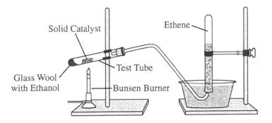
Ethene, C<sub>2</sub>H<sub>4</sub>(g) (molar mass 28.1 g/mol), may be prepared by the dehydration of ethanol, C<sub>2</sub>H<sub>5</sub>OH(g) (molar mass 46.1 g/mol), using a solid catalyst. A setup for the lab synthesis is shown in the diagram above. The equation for the dehydration reaction is given below.
