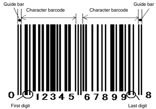
Print result of UPC-A of UPC-A barcode command <BL> followed by <character type> data
