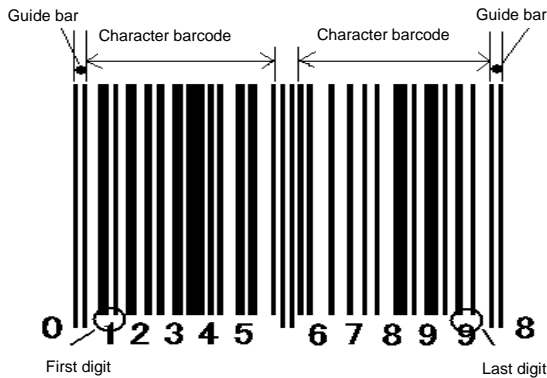
Print result of UPC-A of barcode command <D> followed by <character type> data
