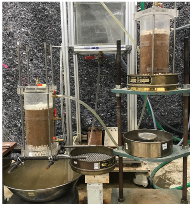
Figure 4. 4 Suffusion test apparatus
