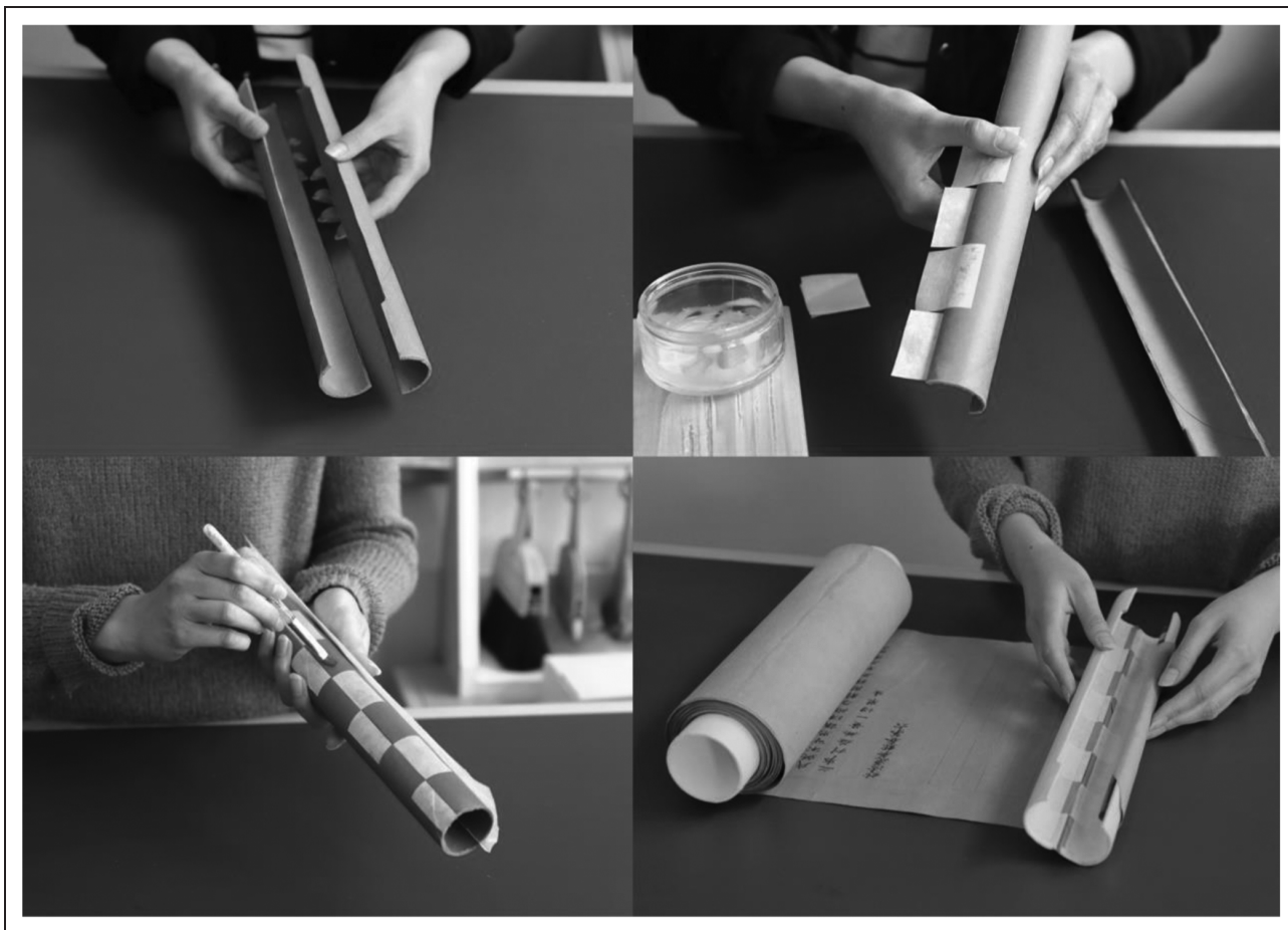
Figure 6. Making a reduced-diameter clasp core.
