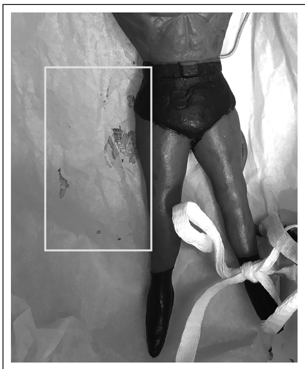
Figure 3. The rectangle highlights plasticizer stuck to the packing tissue.
