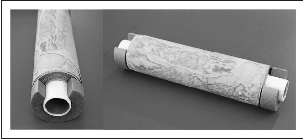
Figure 8. Scroll supports made from polyethylene foam tube and positioned at either end of a 3.5 cm diameter core.
