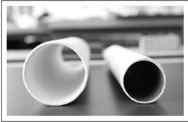
Figure 3. A standard 5.5 cm diameter core outsourced from conservation suppliers (left) and a 3.5 cm reduced-diameter core handmade by International Dunhuang Project conservators (right).
