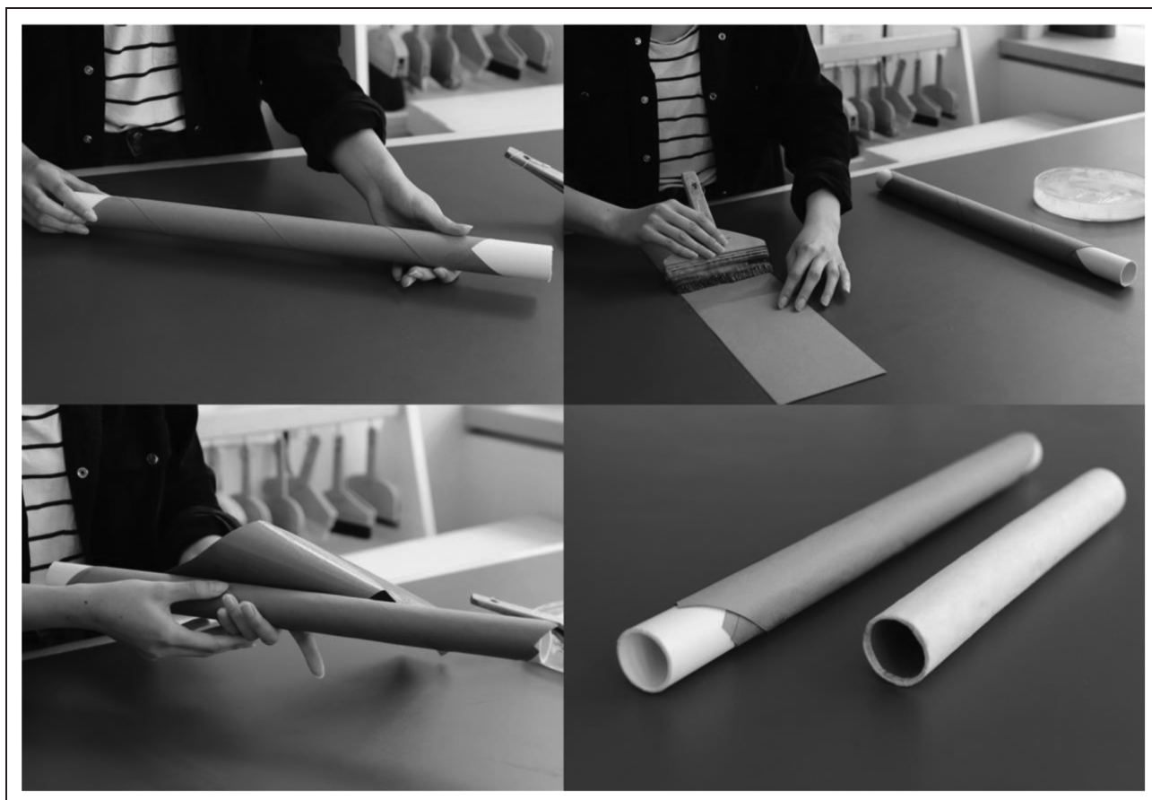
Figure 4. Making a reduced-diameter core.
