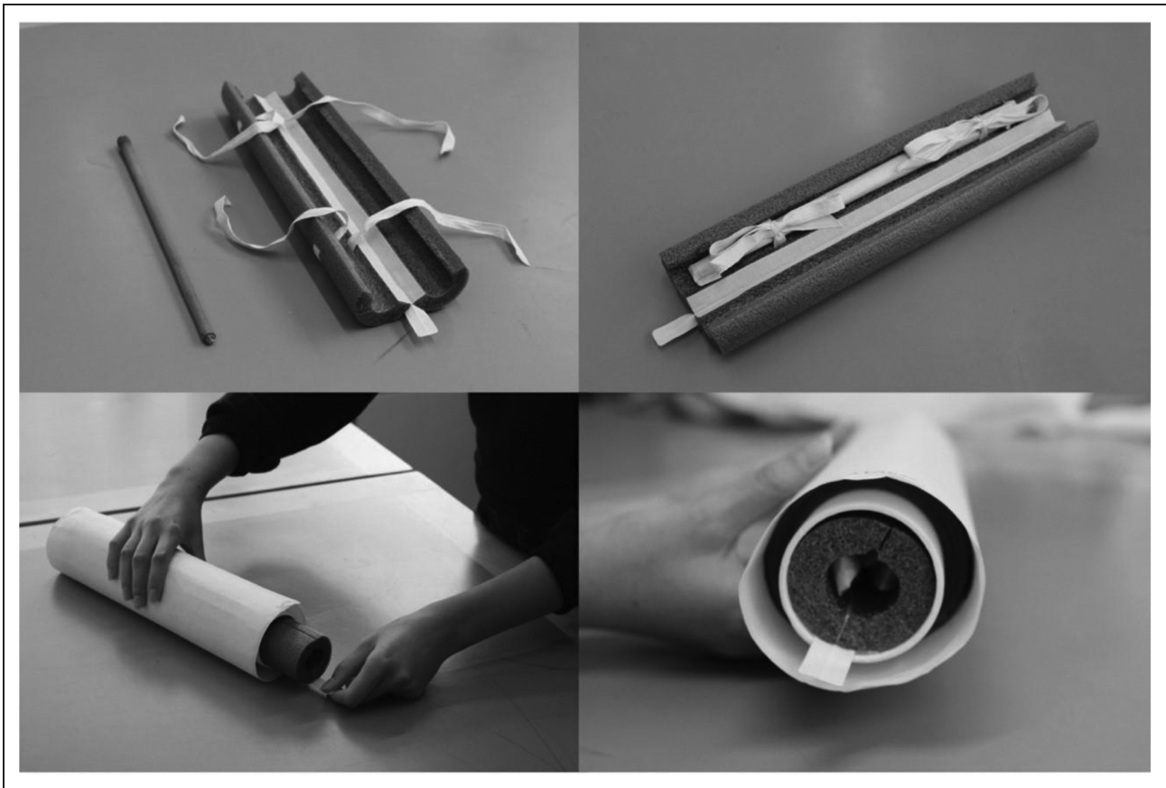
Figure 7. Housing for a detached original roller made out of polyethylene foam tube and stored within a standard core.
