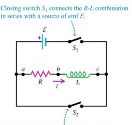
Closing switch  $S_2$  while opening switch  $S_1$  disconnects the combination from the source.
