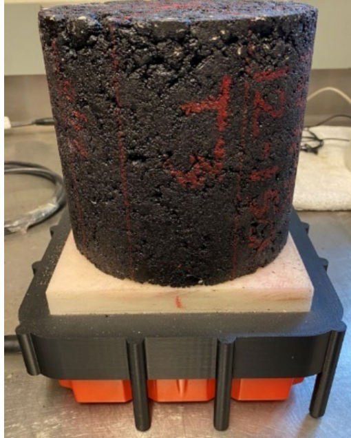
FIGURE 1 Photo of the LDMS setup showing a gyratory compacted asphalt specimen
