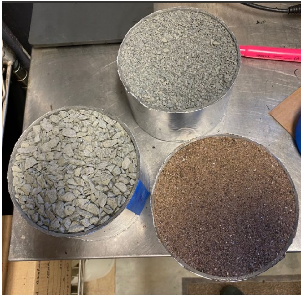
FIGURE 14 Example of compacted specimens of individual component materials
