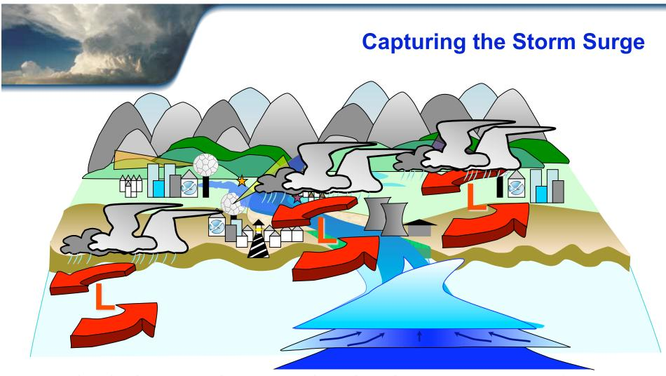
CI-FLOW Ocean Model Suite Provides Storm Surge Simulations (Water Levels) for coastline and for coastal streams, tidal creeks, and bays-
