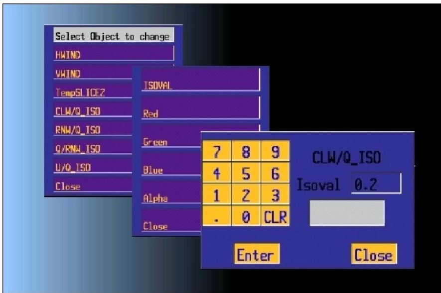
Fig. 2. These panel menus were added to Cave5D to increase its functionality. In this example we are going to modify the value of the cloud water isosurface.
