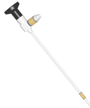
CAD model of a tracked endoscope using custom coil designs
