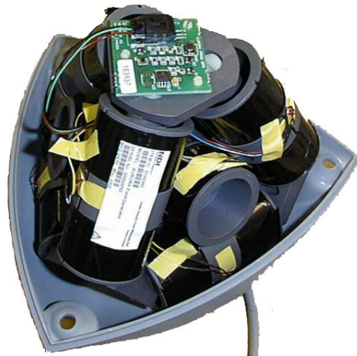
Photograph of the corresponding coils in the Aurora field generator
