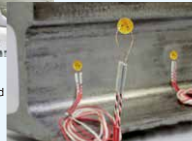
Railway axle load measurement
