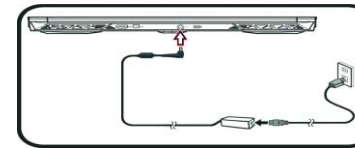
Figure 1 Opening the Lid/LCD/ Computer with AC/DC Adapter Plugged-In
