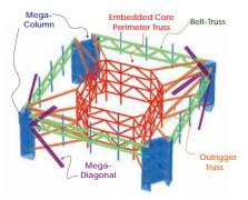
OUTRIGGER TRUSSES Figure 5. Outrigger trusses tie columns, diagonals and belt trusses to the concrete shear walls of the service core.
