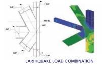
Figure 7. Finite element analysis of a mega-column to megadiagonal connection.
