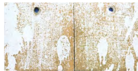
Figure 5. Malaysia: Commercial exterior acrylate paint; Orientation: 60° south facing; Duration: two years
