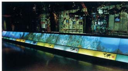
For the videowall, the playback of 18 synchronized video channels is by two servers locked together. The video projectors are a mirror version of the Electrosonic PROVIEW, with diffuser screens to give wide viewing angles. In all there are 72 channels of MPEG-2 video played from Electrosonic servers in the Hall of Biodiversity.
