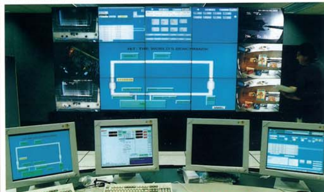
At the Arnold Air Test Facility in Tennessee a 5x3 graphics and video wall display is used to show a mixture of engine test data and video surveillance. Electrosonic ProDigital 40 inch DLP displays with VECTOR processing make up the display.
