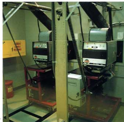
One of the 13 projection systems installed at Spider-Man. 25 70mm projectors are used in all, 23 of which are 8 perf pulldown.
