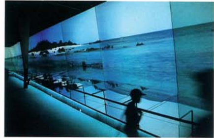
The Venezuela Pavilion at EXPO 98, Lisbon, Portugal used big screen video projection to great effect. Sono-RGB of Barcelona (Electrosonic distributors in Spain) engineered the system and produced the programmes. Projection was by JVC-Hughes ILA™ projectors, and show control by Electrosonic ESLINX.
