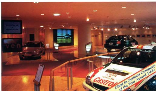
Ground floor view of Le Rendez-vous Toyota. The 3x3 videowall uses Electrosonic VECTOR™ processing and Toshiba "cubes". All exhibition video is fed from Electrosonic video servers - but for special events there is provision for off-air, satellite, VCR and internet sources as well.
