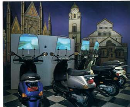
In "Italy" at Vinopolis you ride through the Italian countryside on a "Vespa". The windscreen becomes a viewing screen for a projected video. It uses a PDL screen laminated into the real windscreen (see "Floating Image" story on Page 4 for more about PDL).
