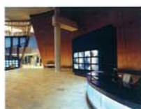
The "Video Aquarium" at the Children's Medical Center, Medical College of Georgia (above) has a counterpart in the "Echo" videowall across the lobby (right). Both displays use Dotronic 27 inch videowall monitors and Electrosonic PICBLOC-3™ processing. Videowall programming by Fury 13.
