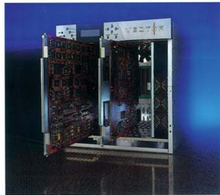
The VECTOR processor, as used by Best Buy, is modular, and can be configured with a variety of input and output cards to suit a wide range of analog and digital inputs and outputs. While mainly intended for videowall use, it is also suitable for multi image processing onto a single screen.
