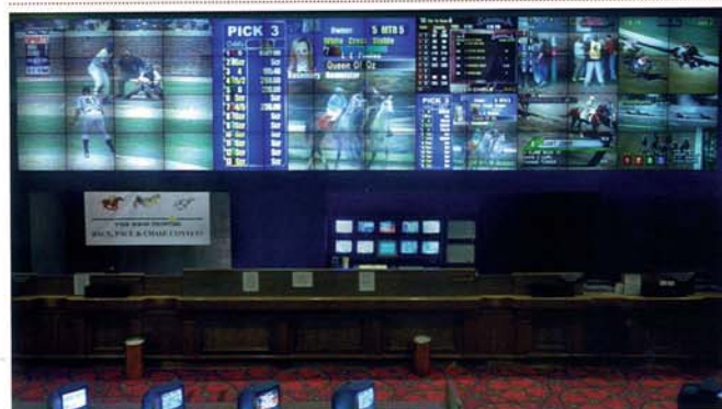
The Sports Book at The New Frontier Casino, Las Vegas, uses a 14x4 Electrosonic videowall. All images are video based, and are predominantly related to horse racing, but also cover all major sporting events. Installation and system design by Diversified Video Inc.
