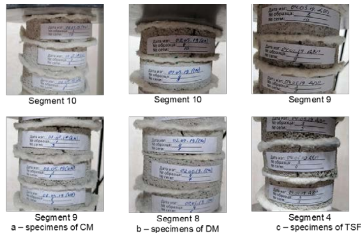
Figure 5. Weakest segments of specimens.
