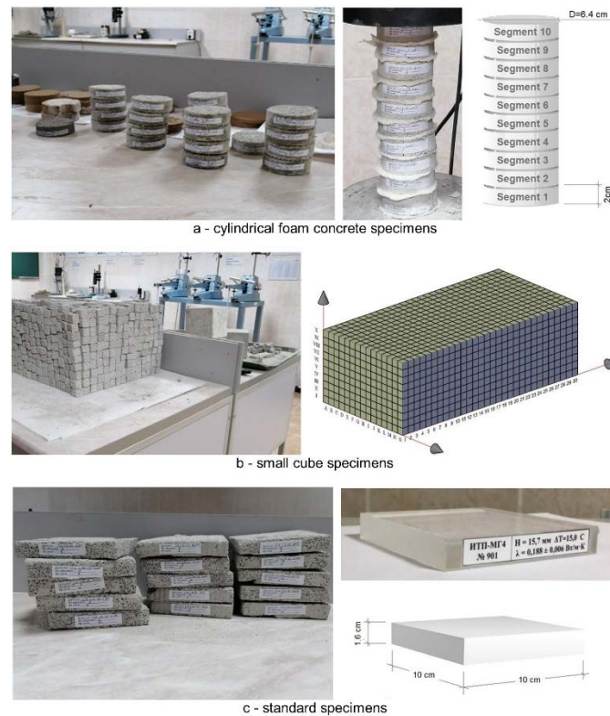
Figure 2. Specimens for determining the physical-mechanical properties of foam concrete.
