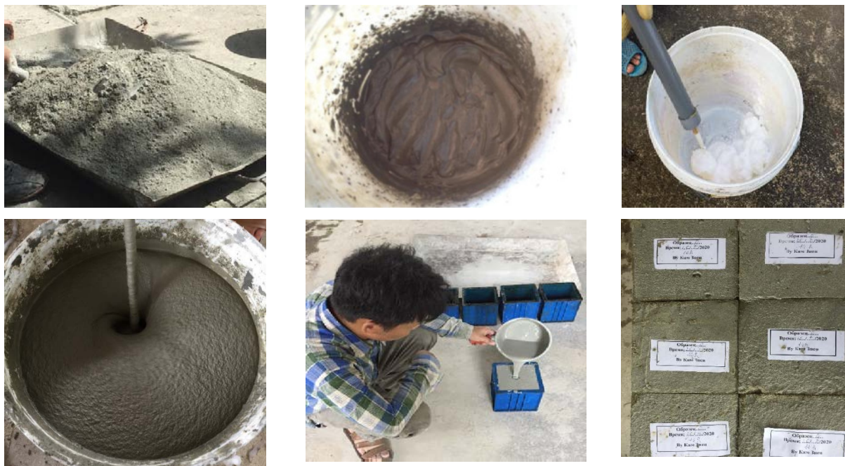
Figure 2. The process of preparing foam concrete samples (from left to right, top to bottom).
