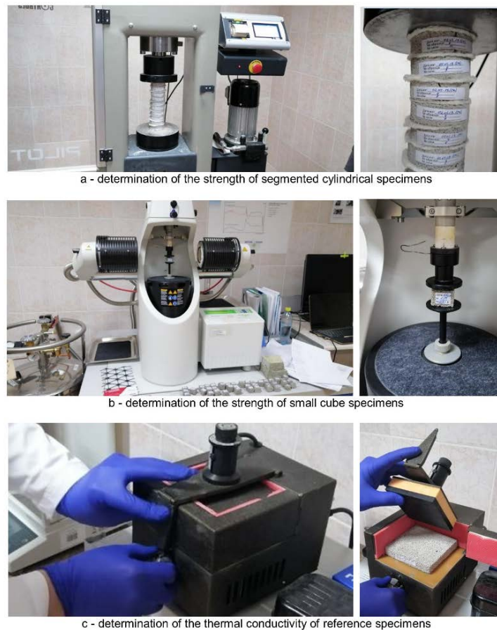
Figure 3. Laboratory testing of foam concrete specimens.
