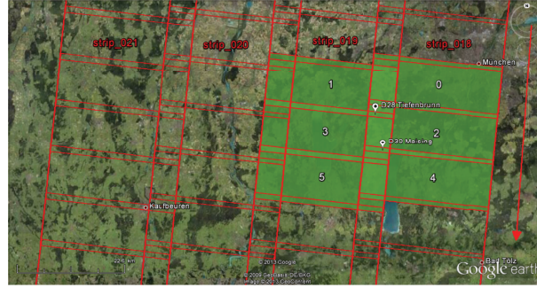
FIGURE 2: TSX TOPS acquisition coverage with subswaths and bursts indicated. The target position and burst labeling are also shown. The arrow indicates the flight direction (Google Earth).
