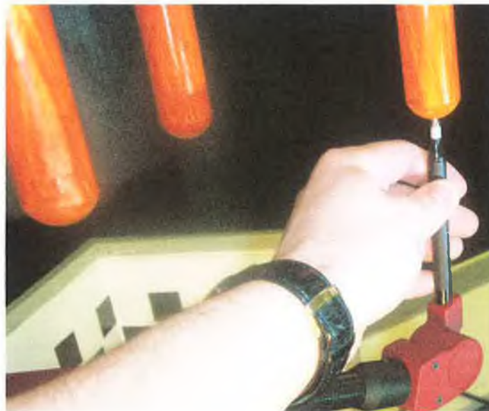
Fig 3.38 – Manually locating the tip of scribe to the guide hole in the teat
