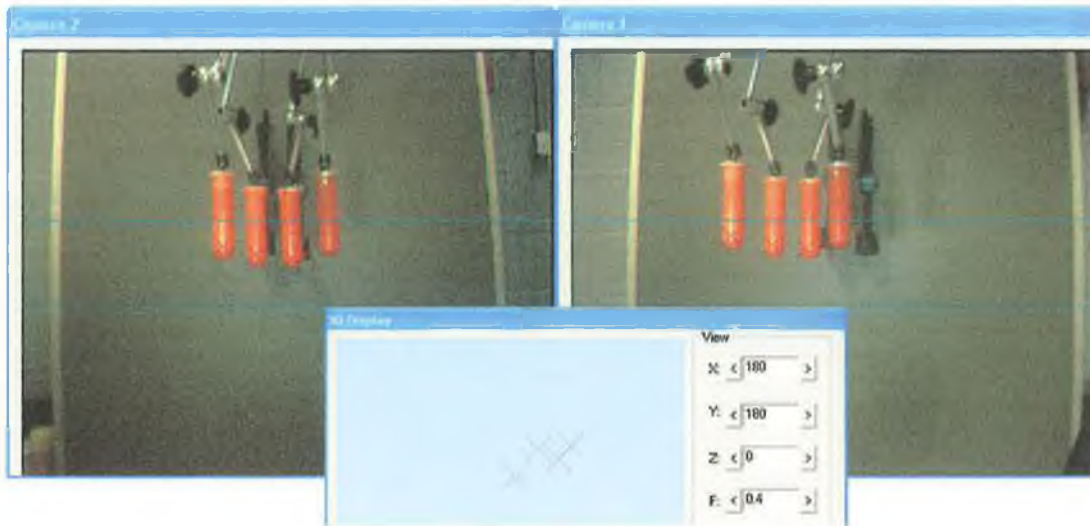
Fig 3.20 – Two teat shaped objects outside of target region – false correspondence between objects
