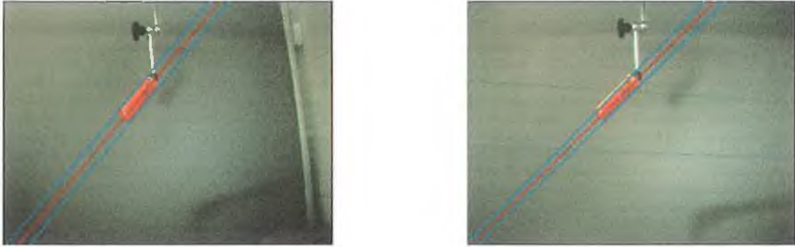
Fig 6.7 – Centerlines in images of Test #11, input = 4px right, 7px down
