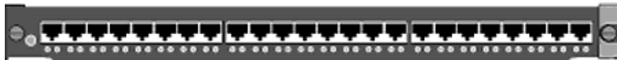
24 port 10/100 Ethernet Line Card with RJ-45 Connectors. (This could be a Fast EtherChannel Card)
