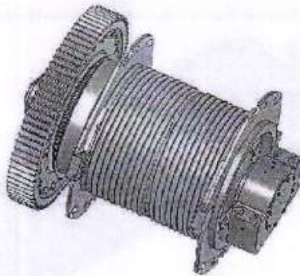
Hoist drum assembly, Alignment is completed with shims under bearing block on RH side.
