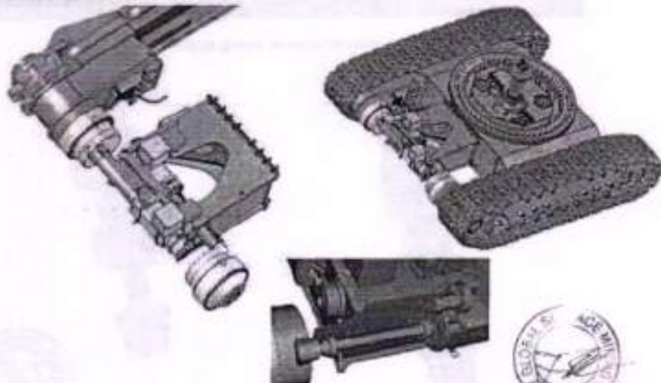
Overall view of propel system with various components removed to show all critical components. No alignment required.
